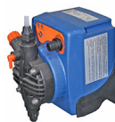
Dosing pump for limestone with electronic control and nitrile seals 5 l/min - 7 Bar Cod. 40.2379.00
